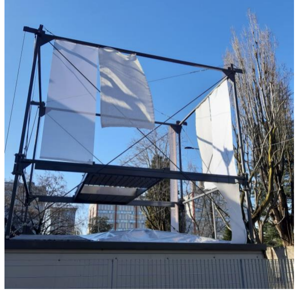
Example of a mesh tested in Rain-Fog Box
