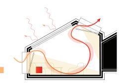
Letting in sunlight for comfort Ventilation for air quality Closing for direct sunlight to not gain heat Ventilate to lower the temperature
